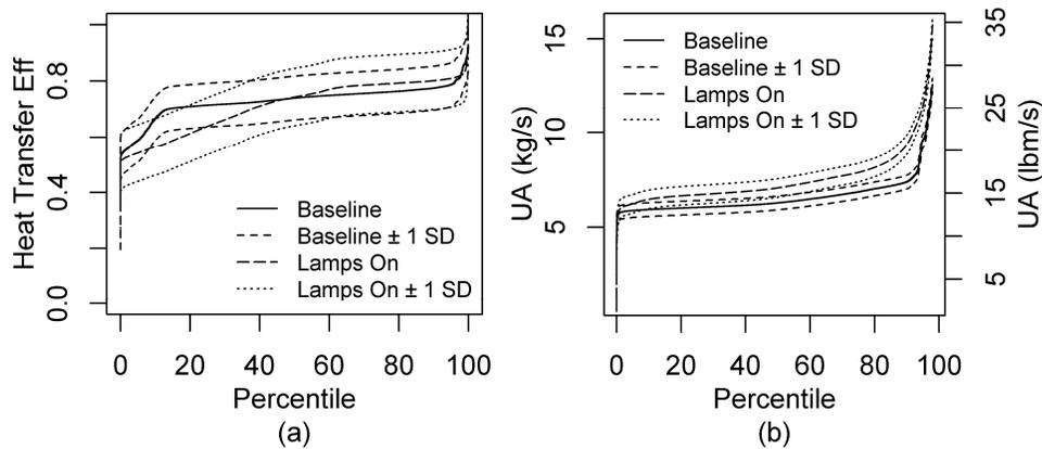
**Figure 2** Cooling Coil Performance (a) effectiveness, value and  $\pm 1$  average standard deviation (b) Heat transfer coefficient at reference point, value and  $\pm 1$  average standard deviation, 98% of values shown for clarity
